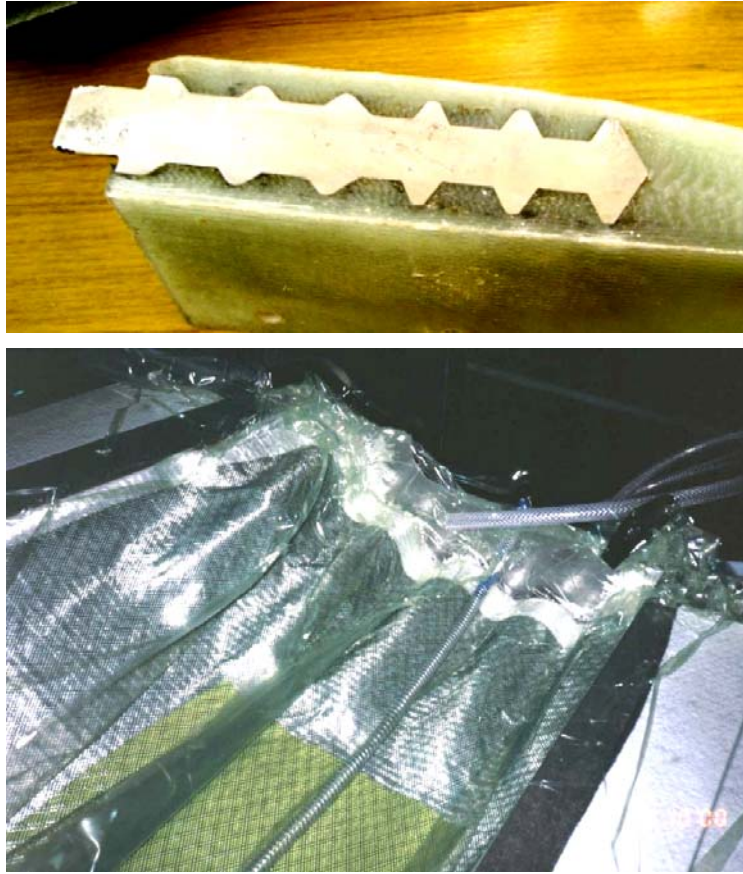
Figure 1 - The 'keyed' root studs used on the new blade: the studs are integrally moulded into the blade root laminate during infusion.
