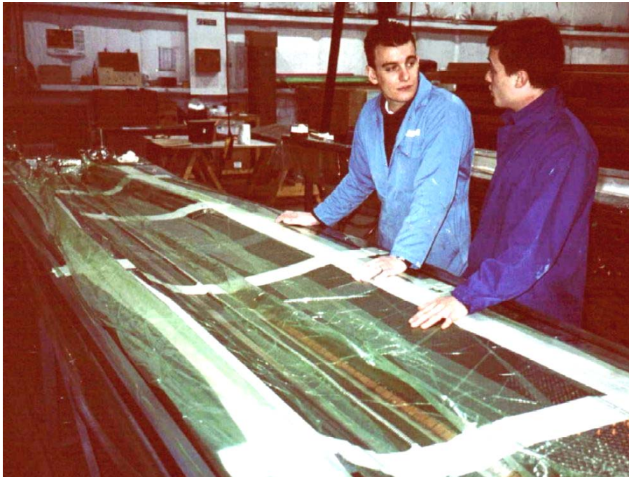
Figure 2 - Infusion moulding of the 7.2m blade: the primary structure (unidirectional glass fibre) is moulded integrally with the blade shell.
