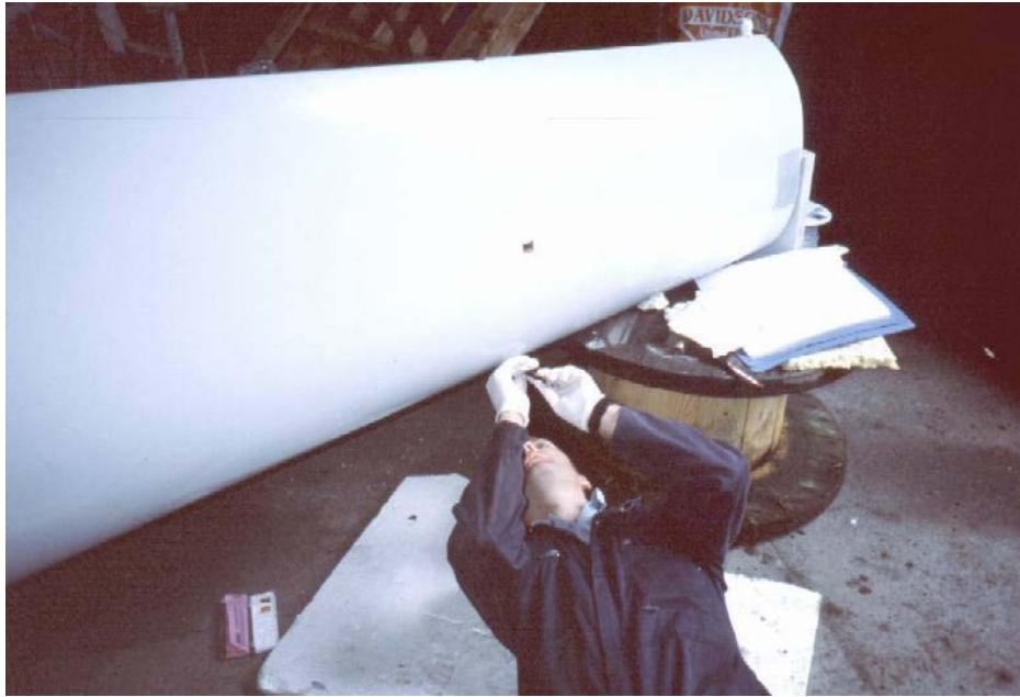
Figure 4 - Attaching strain gauges to the test blade.
